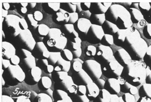
Figure 1 Replica electron micrograph of the clear phase of a 65TeO 2 , 35B 2 O 3 sample etched for 10 sec with a 10% hydrofluoric acid solution, \times 1500 .
