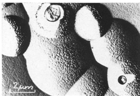
Figure 2 Replica electron micrograph of another region of the same sample as in Fig. 1. The larger magnification ( \times 4500 ) enables the general corrosion of the surface to be seen more clearly.
